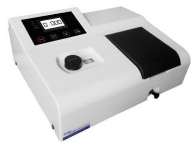
Ringene 752-05 is an (UV-Vis) ultraviolet-visible spectrophotometer used to measure light absorbance across the ultraviolet and visible ranges of the electromagnetic spectrum. When incident light strikes matter it can either be reflected, absorbed, or transmitted. The absorbance of radiation in the UV-Vis range causes atomic excitation, which refers to the transition of molecules from a low-energy ground state to an excited state.
